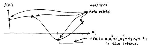
We require that the cubic polynomials have continuous first and second derivatives at the data points marking the point where one cubic polynomial ends and the next begins. This continuity requirement is sufficient to guarantee a unique set of coefficients for the cubic polynomials.
