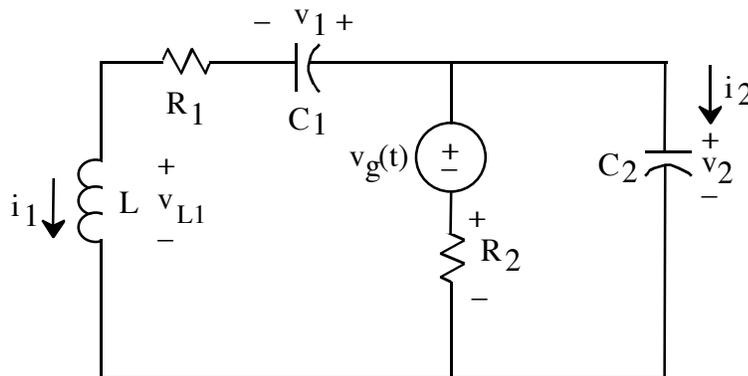
The equation for  $v_{L1}$  must come from a voltage loop, and the voltage loop around the outside will suffice in this case. We use Ohm's law to express the voltages across  $R_1$ .
