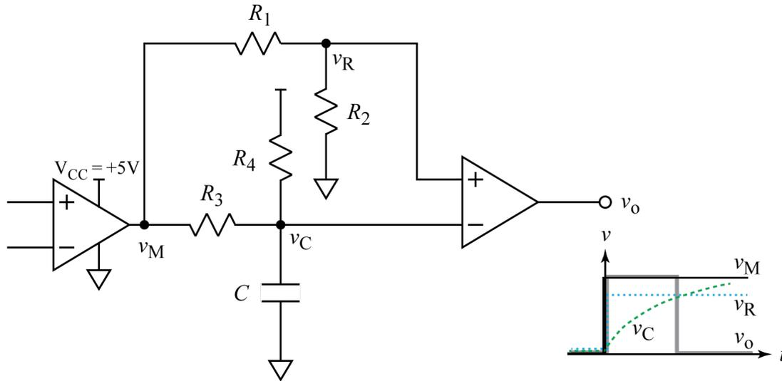
Fig. 1. Pulse generator circuit.
