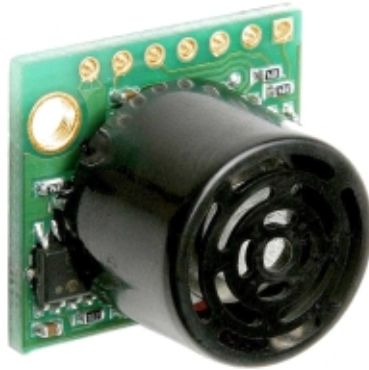
Fig. 2: Picture of the LV-MaxSonar-EZ2 ultrasonic sensor [5].
