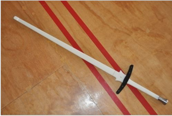
Fig. 4. The base simulator we will use to calibrate and test our smart sword design. This model was originally designed for use in hot, dry climates, as the other models had a tendency to break [8].
