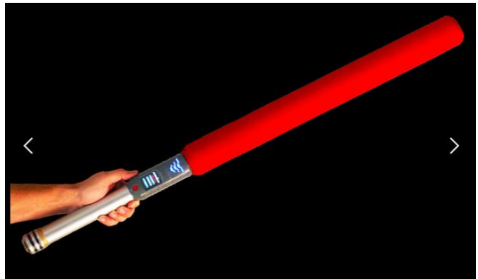
Fig. 1. A one pound foam sword with electronic scoring using accelerometers, Bluetooth, and a touchscreen [4].
