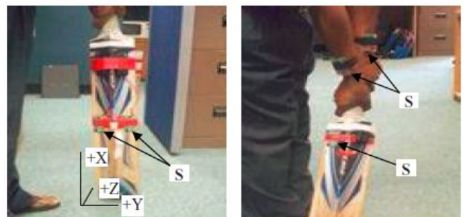
Fig. 2. Accelerometer locations for cricket bat "sweet spot" tests [5].
