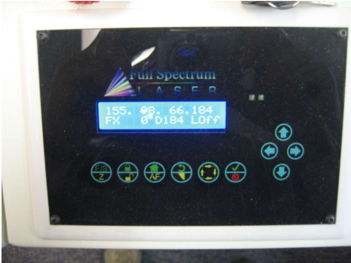
Figure 6: Laser cutter front panel when booted. This shows the default IP address, and that the cutter's control panel is in "Fast XY" (FX) mode. This means that the arrow keys move the laser cutter head in the XY direction. This mode is useful for positioning the head on the cutting bed.
