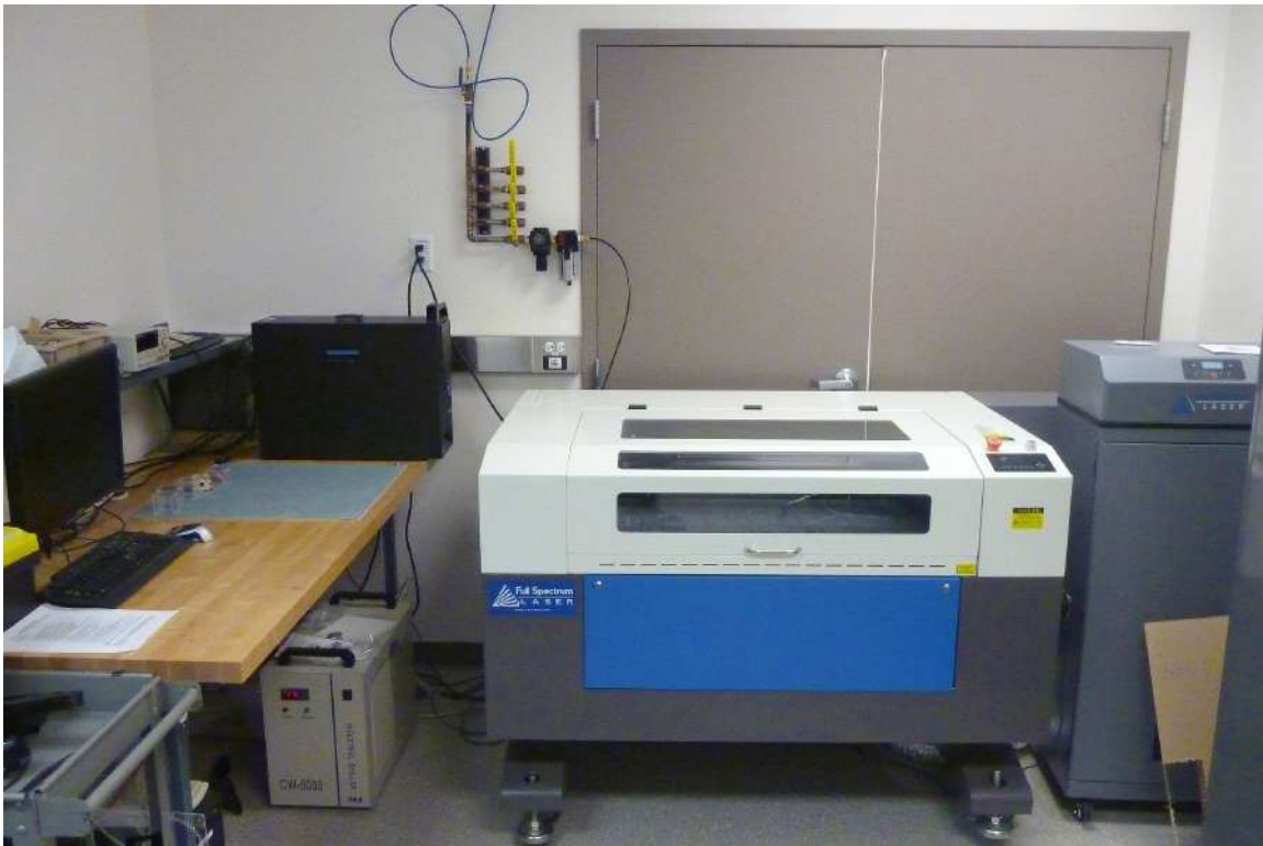
Figure 1: The laser cutter in the Senior Hardware Lab. The water chiller is on the floor to the left. The filter is the grey box on the right. The compressed air is accessed through the manifold on the wall. The black PC is the driving PC.
