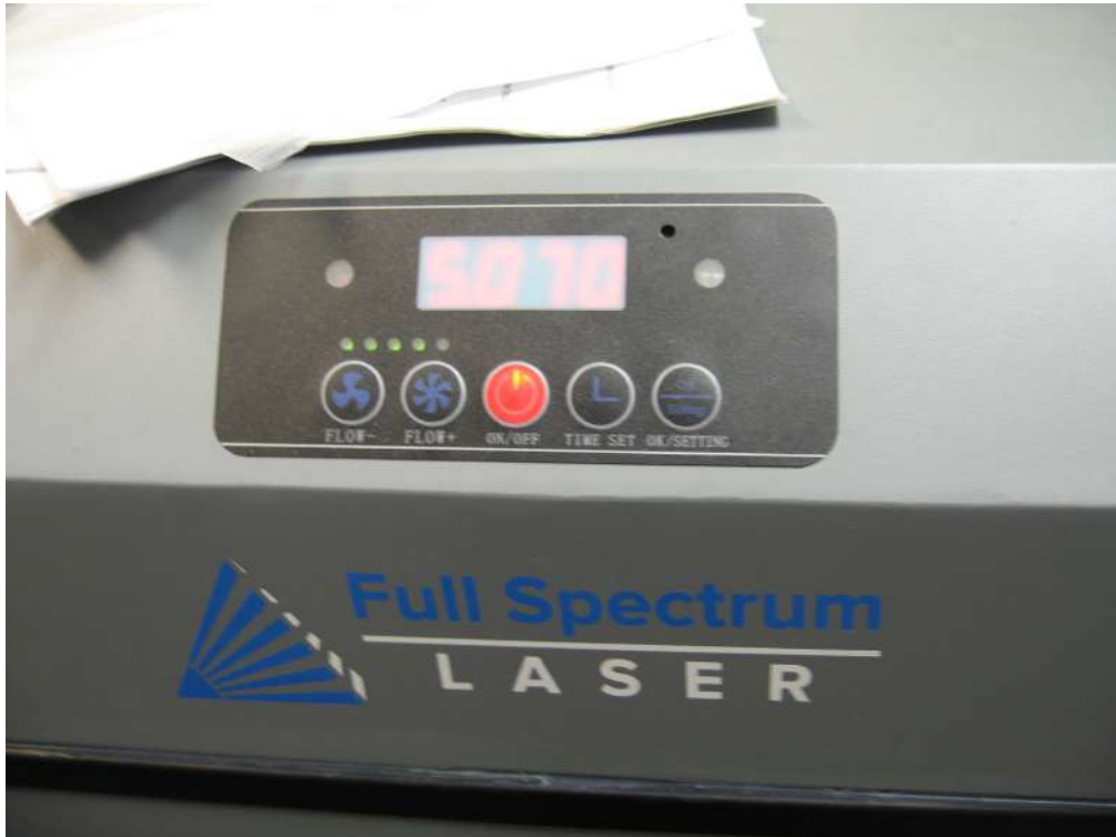
Figure 4: Air filter - up and running at 70% speed (which should be fine for our laser cutter).
