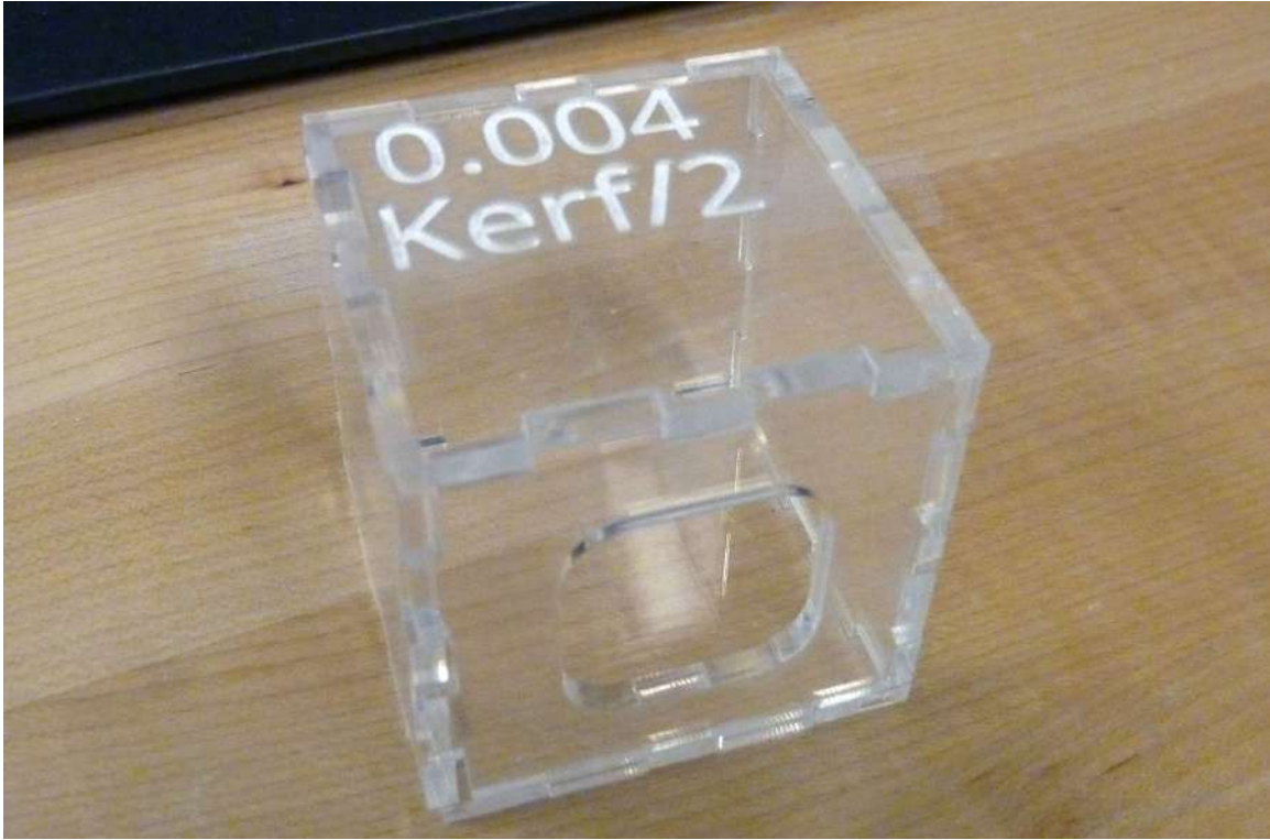
Figure 16: The resulting box held together with friction-fit finger joints.
