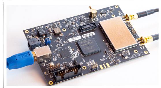
Figure 3. The bladeRF is the RF emitter for the EWS. [6]
