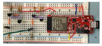
Fig. 5: Level shifting circuit for UART communication between ESP32 and Arduino Mega 2560[4]
