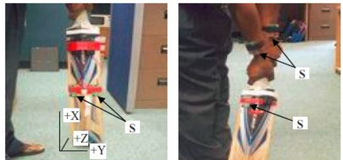
Fig. 4. Accelerometer locations for cricket bat "sweet spot" tests [5].
