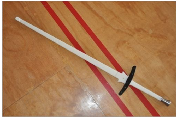
Fig. 8. The base simulator we used to calibrate and test our smart sword design. This model was originally designed for use in hot, dry climates, as the other models had a tendency to break [7].
