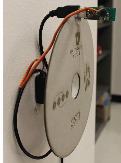
Fig. 1. Rotating Servo-node Platform. The automated prototype used in this work is composed of a TI CC2531 RF sensor, operating in the 2.4 GHz ISM band, and a servo motor that can rotate one full turn (360 degrees). The RF sensor is glued on a rigid cardboard disc having a 10 cm radius. The disc is in turn glued on the winch of the servo motor. The sensor controls the position of the servo motor through one of its I/O ports.
