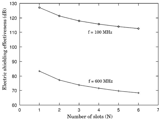
Fig. 3. Electric shielding effectiveness at the center of rectangular cavity with multiple slots as a function of the number of slots;  $a = 1$  cm,  $T_a = 3a$ ,  $\alpha = 20$  cm,  $h = 50$  cm,  $d = 0.4$  cm,  $\theta = 0^\circ$ .
