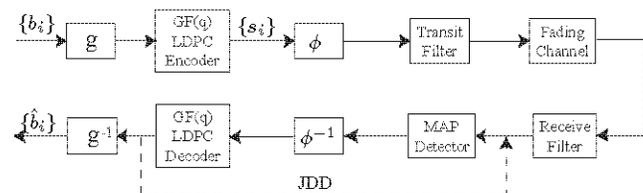
Fig. 1. A schematic block diagram of JDD system.
