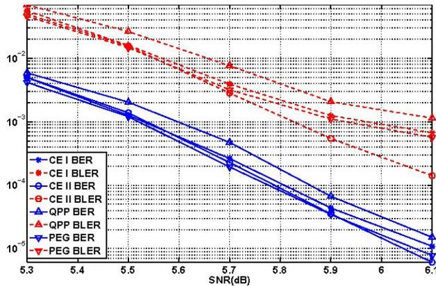
Fig. 3. Performance comparisons of LDPC codes over GF(16) based on CE, QPP, and PEG constructions
