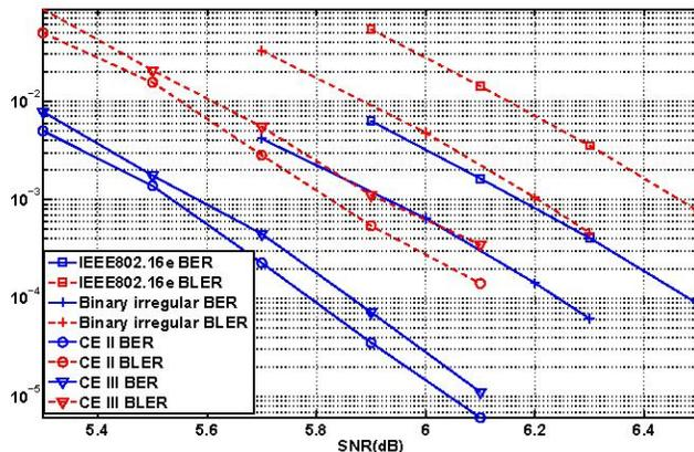
Fig. 4. Performance comparisons nonbinary and binary coded system
