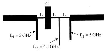
You should have the electrical design finished before coming to Lab, and then use LINECALC to find the line dimensions and ADS to simulate the filter response. We will try to use optimization on this filter to sharpen its cutoff performance at the critical frequency.
