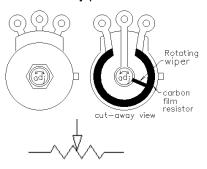
The resistance of a pot is the full resistance between the two outside terminals and is usually written on the part somewhere.
