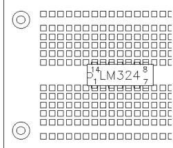
Most op-amp circuits won't work right unless the op-amp is powered with both + and - power supplies. This can be inconvenient, but using op-amps with single-sided supplies is tricky. REMEMBER this! One common mistake people make with op-amps is trying to use them with a single power supply.
