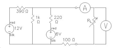
"Zero" both sources, and measure the terminal resistance (R<sub>th</sub>). Make the Thévenin equivalent and confirm the I vs V plot, just exactly like you did before in Experiment 1.
