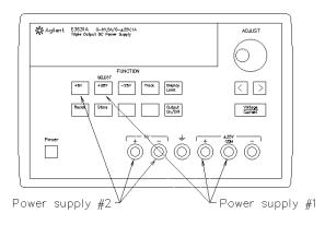
With both power supplies on, the voltmeter should read about 7.2V. Record this voltmeter reading as Vo.
