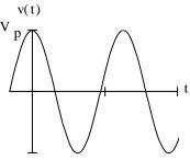
Couldn't we define an "effective" voltage that would allow us to use the same relationships for AC power as used for DC power?
