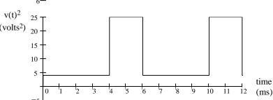
OR...  $V_{RMS} = \sqrt{\frac{1}{T}} \cdot \left[ \int_{0}^{T} (v(t))^2 dt \right]$
