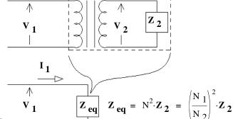
You can replace the entire transformer and load with  $(\mathbf{Z}_{eq})$ . This "impedance transformation" can be very handy.
