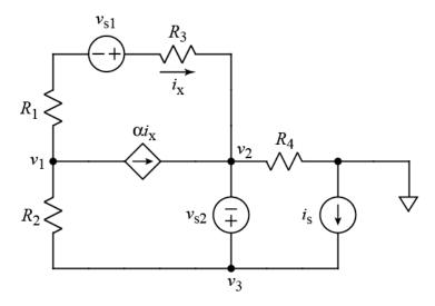
For the circuit shown, write three independent equations for the node voltages  $v_1$ ,  $v_2$ , and  $v_3$ . The quantity  $i_x$  must not appear in the equations.
