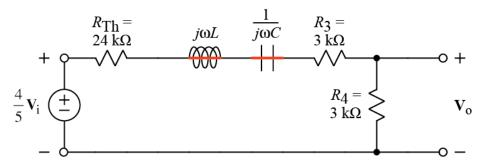
The transfer function is the ratio of the impedance across which  $\mathbf{V}_{\mathrm{o}}$  is measured.
