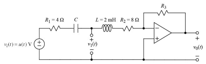
The voltage source in the above circuit is off (0 V) for t < 0.
