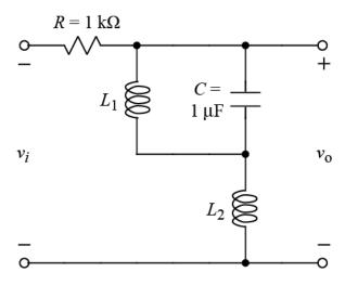
The above filter circuit is intended to be complimentary to the filter designed in ECE 2240 Lab 4. That is, it is designed to have low gain at frequencies where the filter in Lab 4 had high gain, and vice versa.
