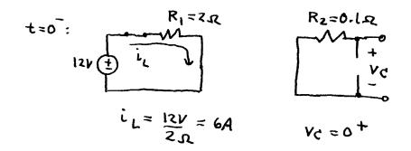
At  $t=0^+$ , we can model the L and C as sources, since  $i_{L}(0^+)=i_{L}(0^-)$ ,  $v_{C}(0^+)=v_{C}(0^-)$ , and any component whose i or v is known may be replaced by a source with that i or v value.
