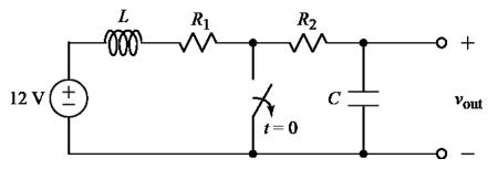
A 12 V power supply drives a long wire, (modeled as L and  $R_1$ ), followed by a short wire,  $R_2$ , and a smoothing capacitor, C. There is a safety switch, located before the smoothing capacitor, to turn off the output at the remote end. The switch is closed for a long time before opening at t = 0.
