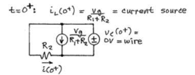
Because the C acts like a wire, all the current from the L will flow thru the C. So the current in  $R_2$  is zero. (Another way to see this is to observe that  $R_2$  has  $OV = V_C$  across it, and by Ohm's (aw  $i(O^{+}) = OV/R_2 = OA$ .)
