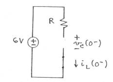
Because of the open circuit,  $i_{\perp}(0^{-}) = 0 A$ and there is no v-drop across R. Thus, the GV is dropped across the open circuit, C.
