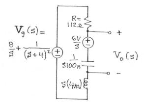
Note: The 6V initial conditions for C must s be included in Vo(s). c) We may use superposition to calculate V. (3).
