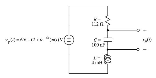
Note: The 6 V in the  $v_g(t)$  source is always on.
