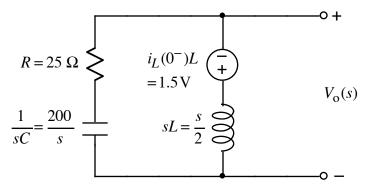
The output voltage is found by using a voltage-divider formula. We observe that  $V_0(s)$  is measured across the *R* and *C*. Thus, we may use a voltage-divider formula that avoids the need to add the voltage source to our answer. (An alternative approach is to use a voltage-divider to find the voltage across the *L* and then add the voltage source to our answer.)
