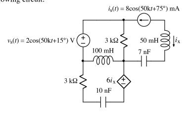
**SOL'N:** In the frequency-domain, we use phasors for voltages and currents, and impedances for resistors, capacitors, and inductors.
