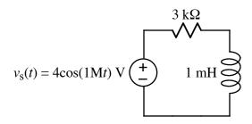
a) Find time-domain expressions for the waveforms of the voltages across the R and L in the above circuit.
