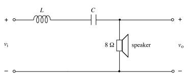
The above circuit is part of a simple crossover network for driving a midrange speaker having an impedance of  $\$\Omega$ . The circuit is described at the following web site: <u>http://www.termpro.com/articles/xover2.html</u>. A more in-depth discussion of crossover networks may be found at <u>http://sound.westhost.com/lr-passive.htm</u>.
