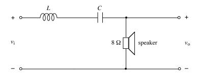
The above circuit is part of a simple crossover network for driving a midrange speaker having an impedance of  $8\Omega$ . The circuit is described at the following web site: <a href="http://www.termpro.com/articles/xover2.html">http://www.termpro.com/articles/xover2.html</a>. A more in-depth discussion of crossover networks may be found at <a href="http://sound.westhost.com/lr-passive.htm">http://sound.westhost.com/lr-passive.htm</a>.
