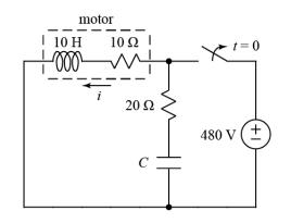
After being closed for a long time, the switch opens at t = 0.
