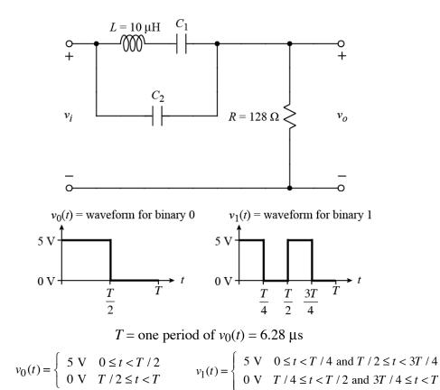
The above filter circuit is being used in a communication system to detect whether received signals represent binary zeros or binary ones. The waveforms are designed to be detected using a method that determines whether the signal is high or low in each segment of length T/4, but only the analog filter circuit shown above is
