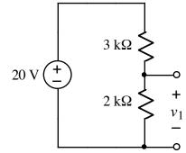
b) Use the voltage-divider formula to calculate  $v_1$ .
