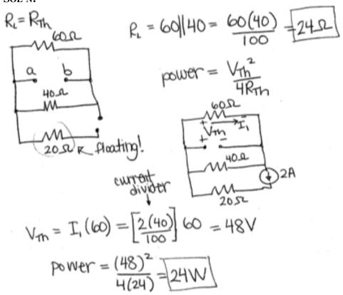
Note: Circuit used to find max power value is shown below.
