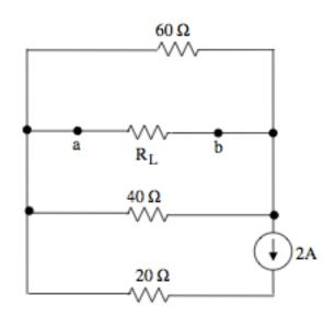
a) Calculate the value of  $R_{\rm L}$  that would absorb maximum power.
