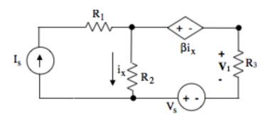
Using superposition, derive an expression for  $v_1$  that contains no circuit quantities other than  $i_s$ ,  $v_S$ ,  $R_1$ ,  $R_2$ ,  $R_3$ , and  $\beta$ , where  $\beta$ <0.
