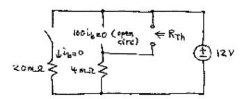
We observe that the Thevenin equivalent seen from the terminals where the L is connected is just the 4ms and 1211:
