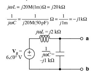
b) The Thevenin voltage is the voltage across a and b with no load attached. We have a simple V-divider.
