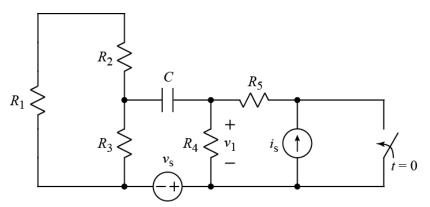
After being open for a long time, the switch closes at t = 0.  $v_s = 28 \text{ V}$   $i_s = 112 \text{ mA}$  C = 2 nF $R_1 = 43 \Omega$   $R_2 = 47 \Omega$   $R_3 = 120 \Omega$   $R_4 = 750 \Omega$   $R_5 = 1 \text{ k}\Omega$
