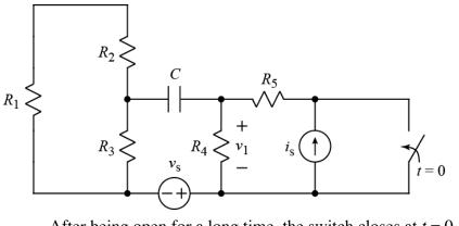
After being open for a long time, the switch closes at t = 0.  $v_s = 28 \text{ V}$   $i_s = 112 \text{ mA}$  C = 2 nF $R_1 = 43 \Omega$   $R_2 = 47 \Omega$   $R_3 = 120 \Omega$   $R_4 = 750 \Omega$   $R_5 = 1 \text{ k}\Omega$
