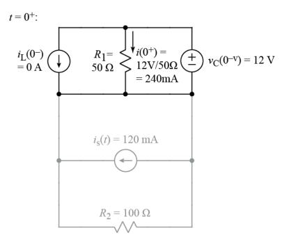
Since the voltage of the capacitor is directly across  $R_1$ , we use Ohm's law to find the initial value of  $i(0^+)$ .
