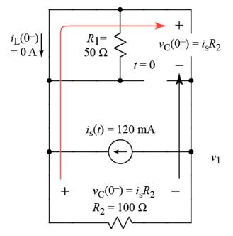
Because of the open circuits, no current can flow in the *L*, so  $i_L = 0$  A. As indicated by the arrows in the above diagram, the voltage drop across *C* is the same as the voltage drop across  $R_2$ , which is  $i_s R_2$ .
