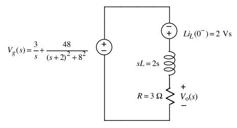
c) We have a voltage-divider driven by the sum of the voltage sources:
