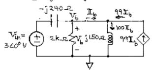
A straight-forward solution approach is to use the node-voltage method with  $V_0$  on the top rail.
