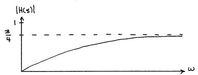
c) The cutoff frequency,  $w_c$ , is the frequency where  $|H(s)| = \frac{1}{\sqrt{2}} \max_{w} |H(s)| = \frac{1}{\sqrt{2}} \cdot \frac{3}{4}$ .
