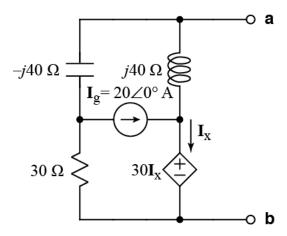
b) We may replace the dependent source with a resistance since we have both the voltage and the current in terms of the current.
