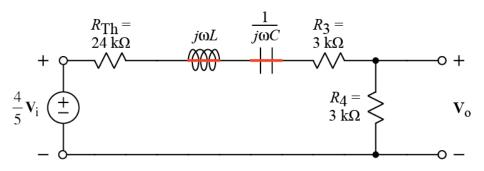
The transfer function is the ratio of the impedance across which  $\mathbf{V}_{0}$  is measured.
