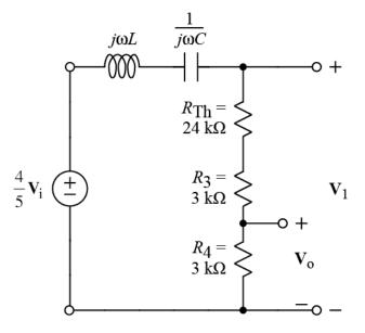
We can express the transfer function in terms of the transfer function of  $V_1$  relative to  $V_i$ .
