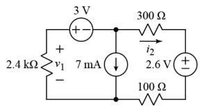
Using the passive sign convention, complete the labeling of all currents and voltages for the resistors in the above circuit.
