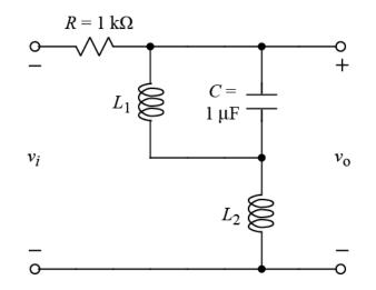
The above filter circuit is intended to be complimentary to the filter designed in ECE 2240 Lab 4. That is, it is designed to have low gain at frequencies where the filter in Lab 4 had high gain, and vice versa.
