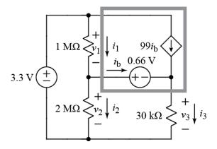
The voltage loops on the left and lower right avoid passing through the current source and yield the following equations when proceeding in a clockwise direction (and using the *v*-drop sign where we exit each component):
