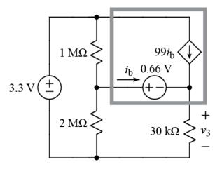
Find  $i_b$ ,  $v_3$ , and the power dissipated by the components in the box.
