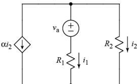
c) Derive an expression for  $i_1$ . The expression must not contain more than the circuit parameters  $v_a$ ,  $R_1$ ,  $R_2$ , and  $\alpha$ . **Note:**  $\alpha > 0$ .
