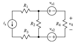
Using superposition, derive an expression for  $v_4$  that contains no circuit quantities other than  $i_s$ ,  $v_{s1}$ ,  $v_{s2}$ ,  $R_1$ ,  $R_2$ ,  $R_3$ , and  $R_4$ .
