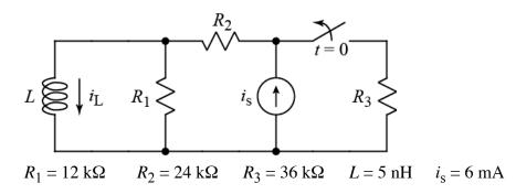
After being closed for a long time, the switch opens at t = 0.
