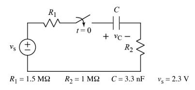
After being open for a long time, the switch closes at t = 0. The initial voltage on the capacitor is  $v_{\rm C}(t = 0^+) = 1.5$  V. Hint: think Thevenin equivalent for the circuit the capacitor is connected to.
