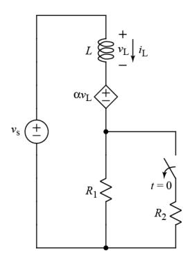
After being closed for a long time, the switch opens at t = 0.
