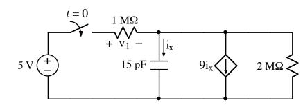
After being open for a long time, the switch closes at t = 0. Find  $v_1(t)$  for t > 0.
